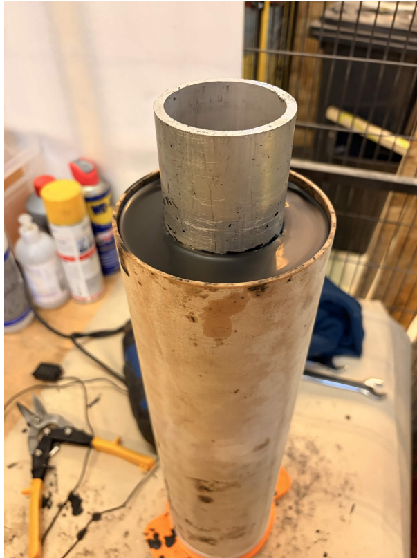
Figure 4.14: Fuel grain manufactured using the vacuum-assisted casting method
