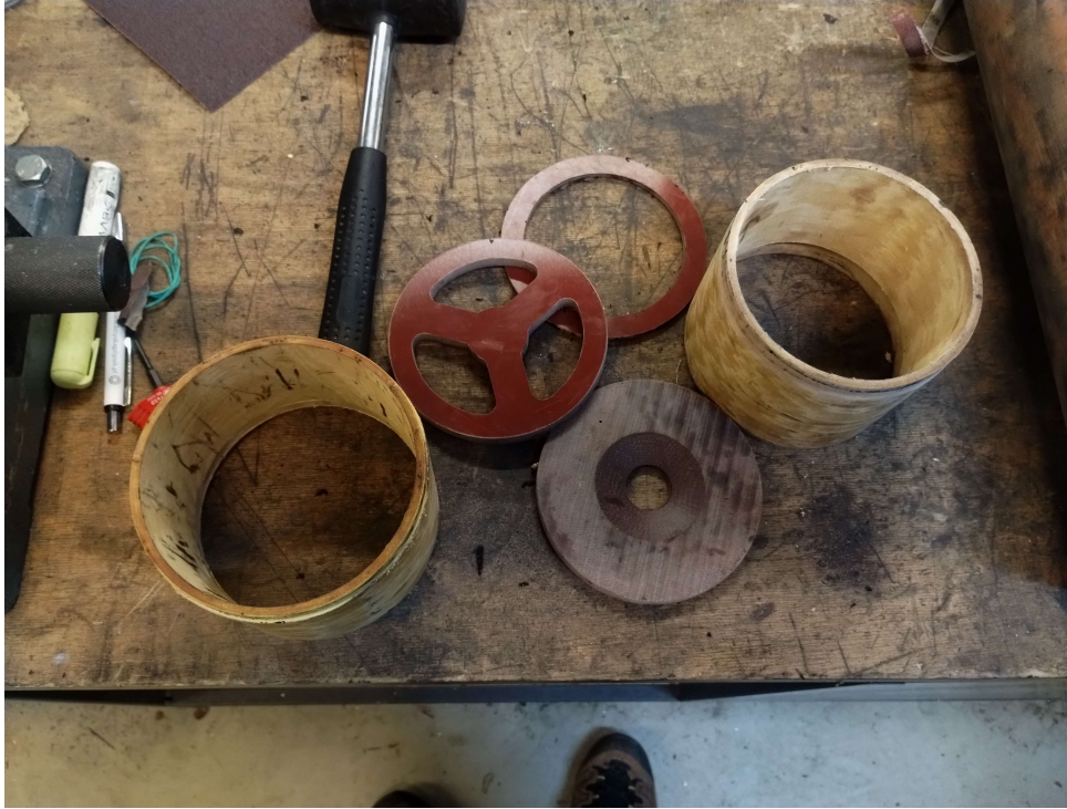
Figure 4.9: Manufactured insulation elements.
