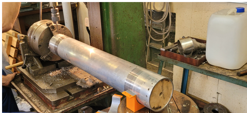
Figure 4.6: Manufactured combustion chamber walls.
