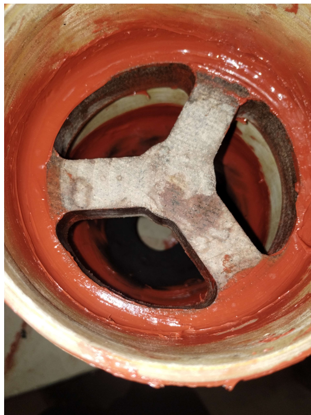
Figure 4.11: Assembled parts with room temperature vulcanizing (RTV) silicone.
