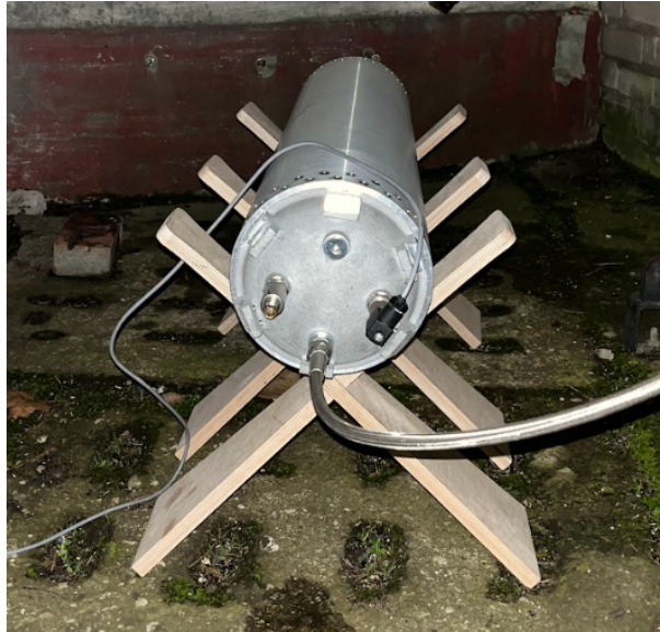
Figure 4.21: Oxidizer tank during hydro-test.
