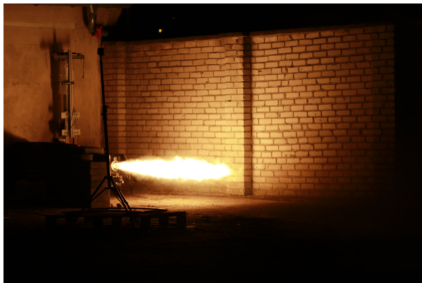
Figure 4.27: 3rd static fire testing
