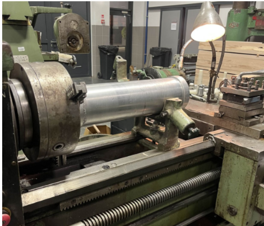
Figure 4.13: Centrifugal casting stand mounted on a lathe.
