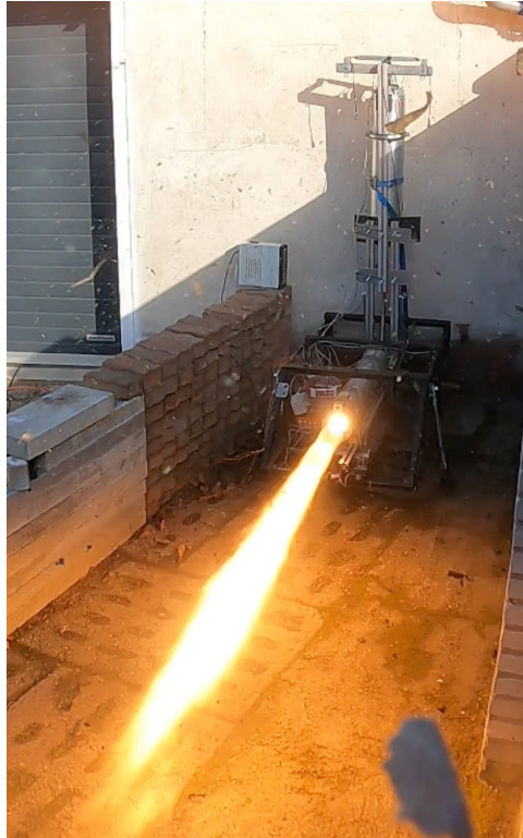
Figure 4.25: 2nd static fire testing
